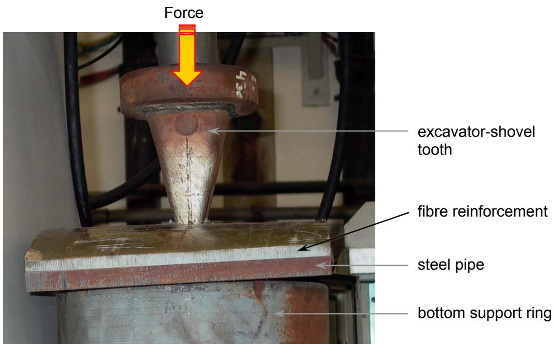
Figure 2: Quasi-static denting test during application of load (excavator-shovel tooth R = 8 mm)
