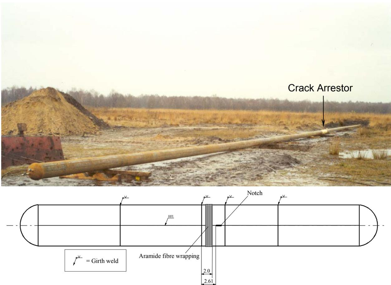
Figure 7: Test setup of the burst test on a HFI pipeline section
