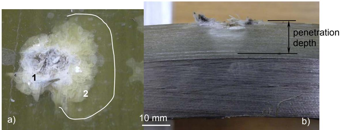
Figure 1: a) Crack arrestor after the ball-impact test showing primary (1) and secondary (2) damaged zone
