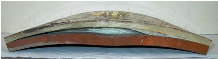
Figure 4: Crack arrestor after the quasi-static denting test
