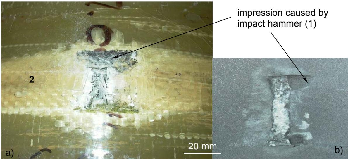
Figure 6: Crack arrestor after the dynamic denting test showing primary (1) and secondary (2) damaged zone; a) Fibre wrap, b) Impression in the outer side of the steel pipe ball-impact test
