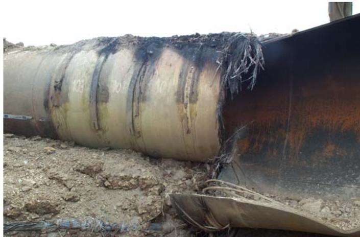
Figure 9: Crack arrestor after the full-scale test
