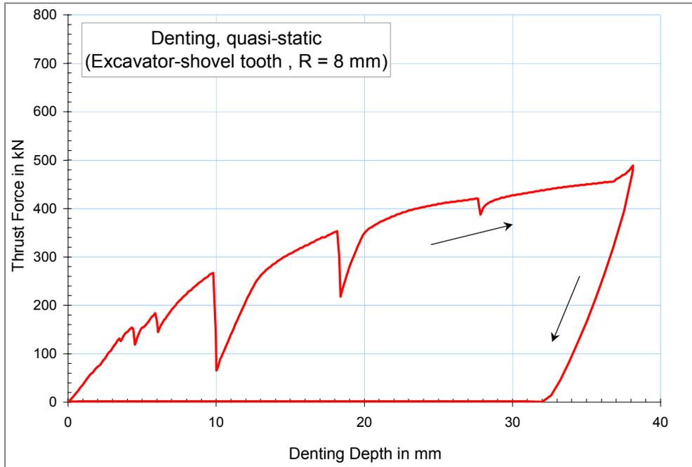
Figure 3: Plot of thrust force as denting depth rises in quasi-static denting test
